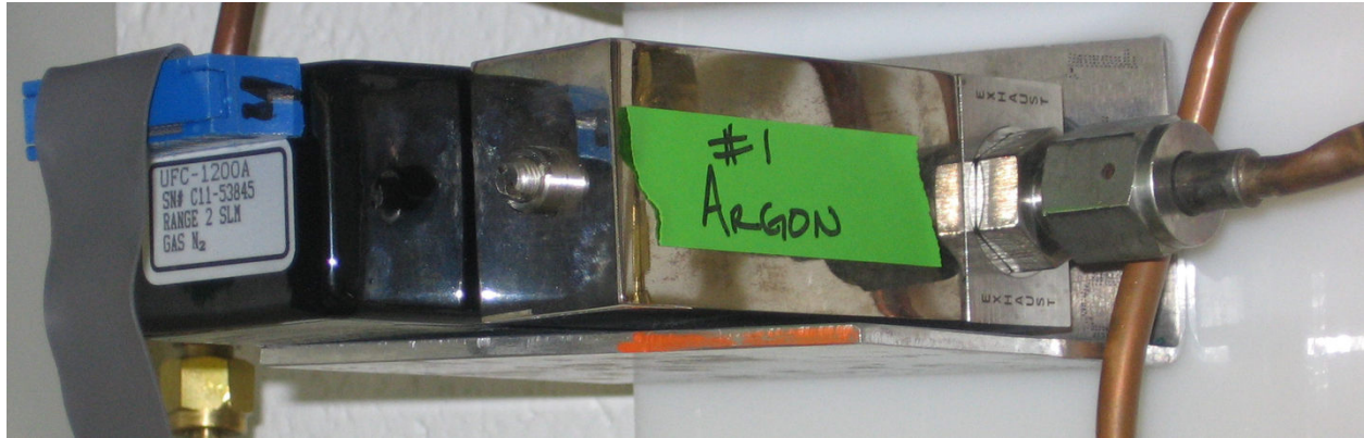
Figure 4.7 Mass Flow Controller used to control the argon flow.
