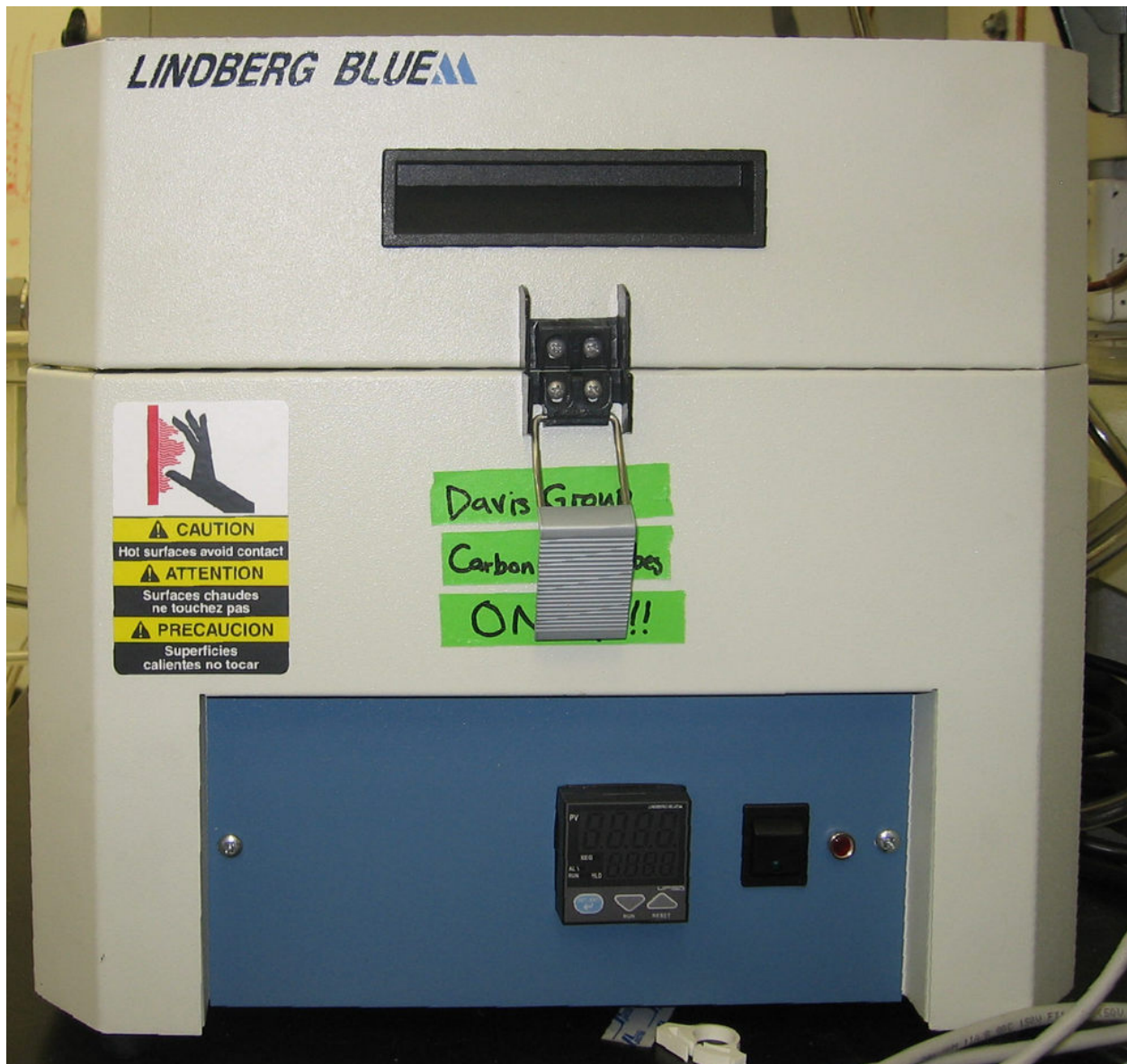
Figure 4.4 Furnace used to perform the argon anneals in.
